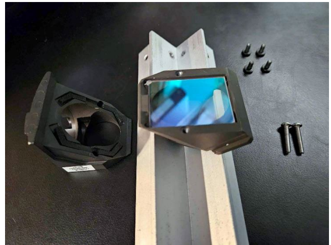
Step 4: Place the beam splitter in the cube with the arrow on the side of the filter point up.
