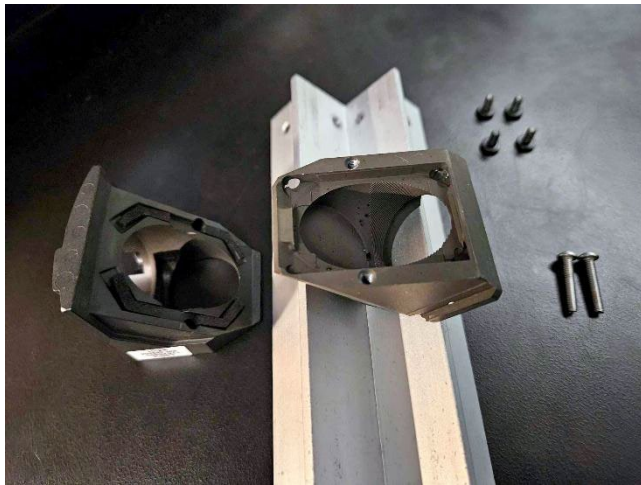
Step 3: Place the cube half with the beam splitter frame on a stable surface to keep the cube level.
