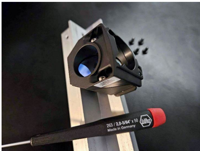
Step 5: Rest the other half the cube on top of the half with the beam splitter, aligning the screw holes. Once aligned, use the hex driver to mount the two longer screws.
