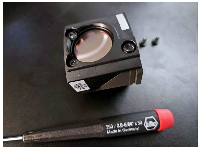
Step 6: The exciter goes in the exciter port on the front of the cube with the arrow pointing in towards the beam splitter. Secure the exciter with two screws.
